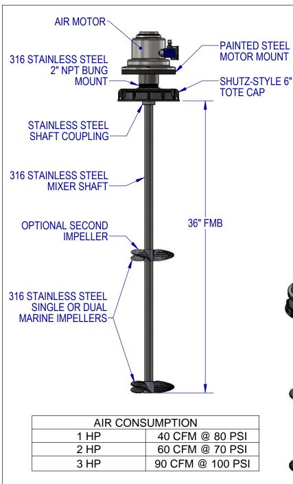
STANDARD FEATURES: PAINTED AIR MOTOR WITH MUFFLER TOTE CAP MOUNT WITH TIE ROD KIT 316SS WETTED PARTS 3/4" X 36" FMB SHAFT SINGLE OR DUAL MARINE IMPELLERS WITH SET SCREW ATTACHMENT SPEED CONTROL VALVE
