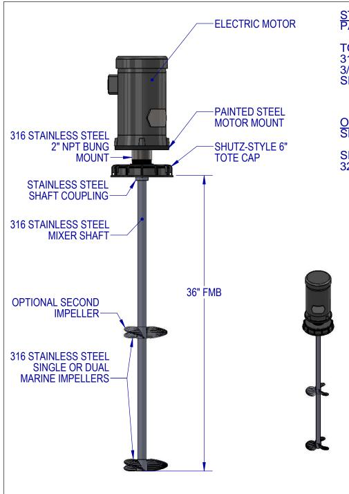
STANDARD FEATURES: PAINTED THREE PHASE, TEFC, 220/440/60 ELECTRIC MOTOR 1750 RPM NOMINAL TOTE CAP MOUNT WITH TIE ROD KIT 316SS WETTED PARTS 3/4" X 36" FMB SHAFT SINGLE OR DUAL MARINE IMPELLERS WITH SET SCREW ATTACHMENT
